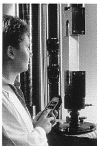
The values achieved for maximum tensile force elongation shows for most specimen that the specific strength of high tenacity chemical fibers is higher than that of conventional building steels.
